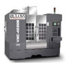
center is a linear guide way machine with a 12,000 rpm spindle with travels of X20.47", Y14.96" and Z13.8". The machine has rapids of 2,362 ipm and a turret type tool changer.
